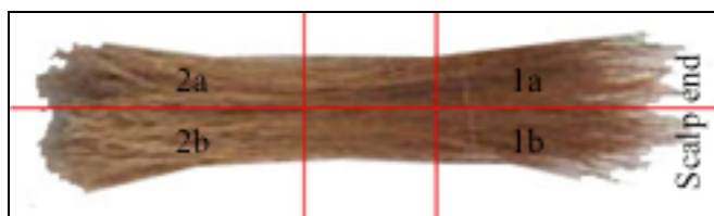
Figure II. Repeatability Sectioning of Hair Sample
