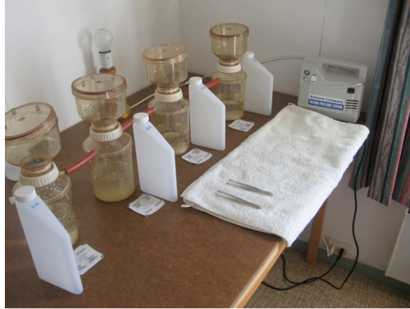
Figure 16: Vacuum filtration lab showing bottles from ISCO water sampler
