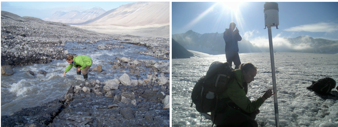
Figure 17: Grab sample being taken at the toe of the glacier Figure 18: Manual ablation readings, HOB0 precip gauge also pictured
