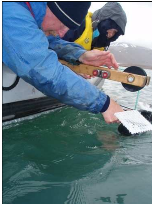
Figure 2.4: The image illustrates the retrieval of the mooring. The pulley assists with the hauling of the mooring and the traps are removed from the line before reaching the pulley. From Cobin, 2008.
