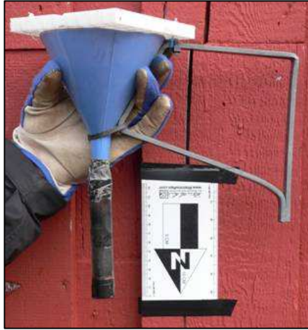
Figure 2.3: Image on the left is the year-long sediment trap complete with funnel, bracket, and receiving tube. Image on the right is the complete spring trap (From Motley, 2006).
