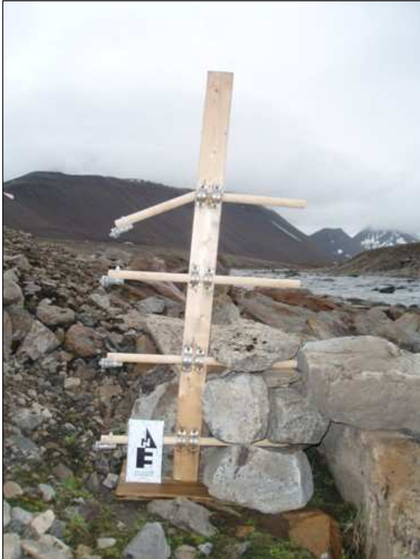
Figure 2.9: The snow tree consists of a two by four stand with rungs attached. The loggers are at 7 cm, 15 cm, 30 cm, and 45 cm from the bottom to the top.
