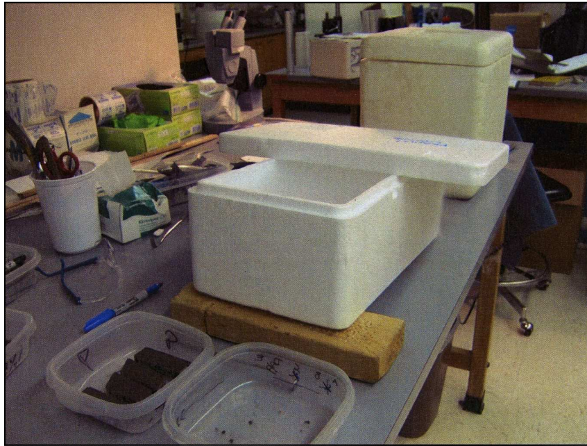
Figure 2.15: The slanted box was used for the liquid nitrogen slow submersion while the standing box was used for complete submersion (From Leon, 2006).
