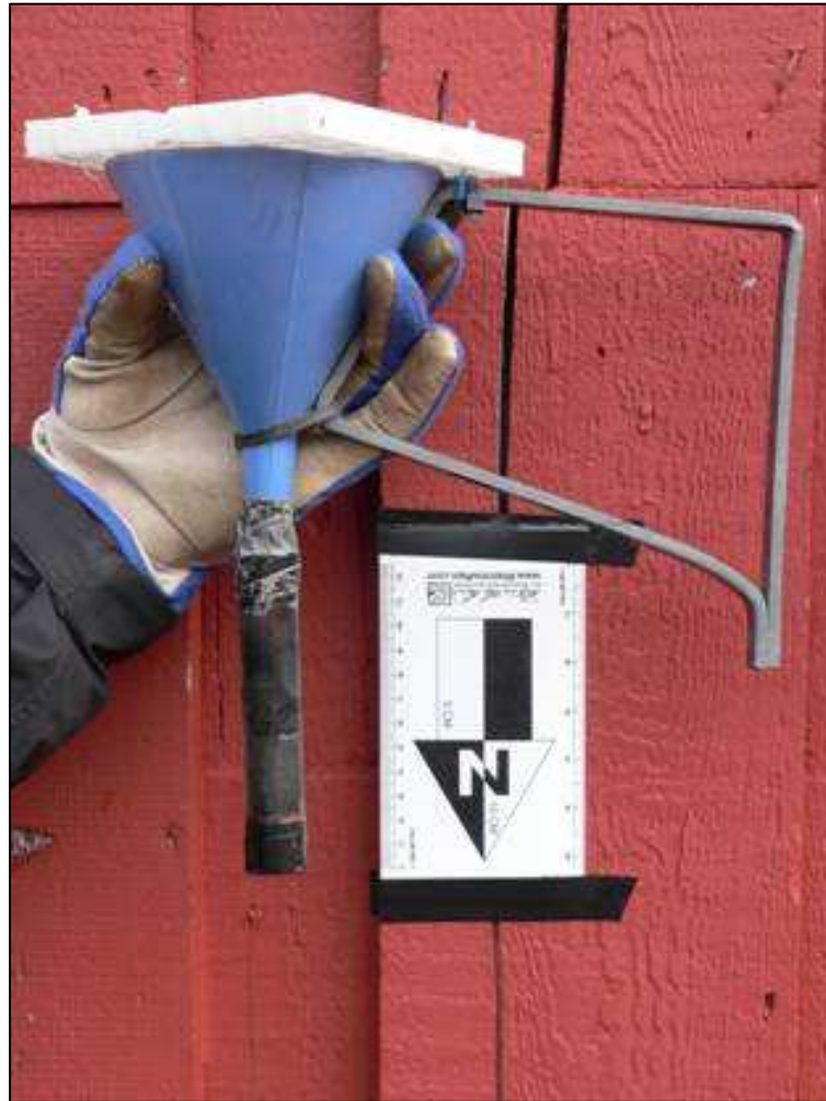
Figure 1.22: Image of the sediment trap model used. The blue funnel is used to capture the sediment and the tubing collects the accumulation. The white baffle is a 1 cm 2 grid and protects the sediment from bioturbation.
