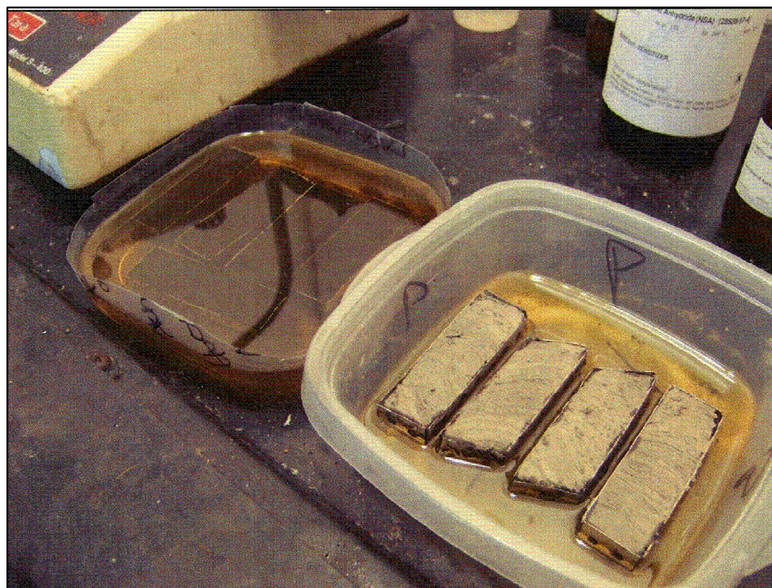
Figure 2.16: This image illustrates the epoxy impregnation. The box on the right has epoxy half-way up the side of the freeze-dried blocks. The box on the left shows the samples fully submerged (From Leon, 2006).
