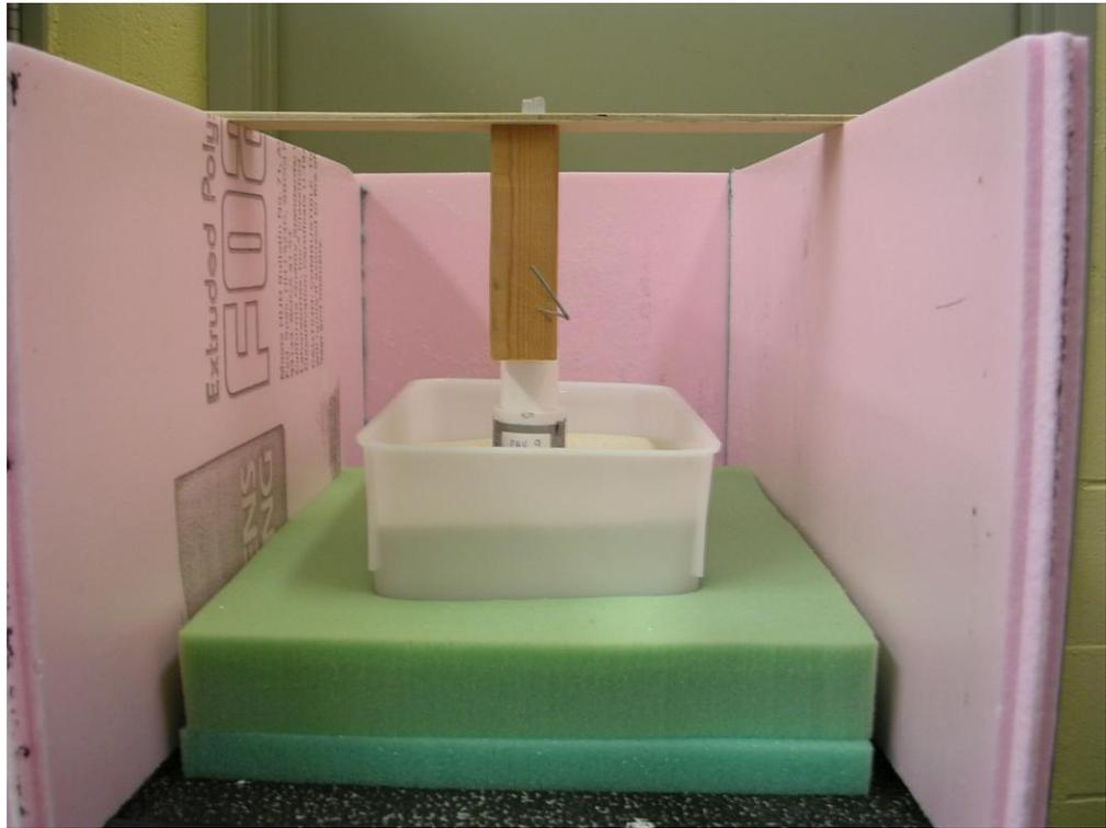
thick) was used to confine each antlion to a small circular area in the center of the plastic container; this procedure ensured that antlions did not build a pit along the wall of the plastic container. Once the pit had been built, the ring was carefully removed so as not to disturb the pit.
