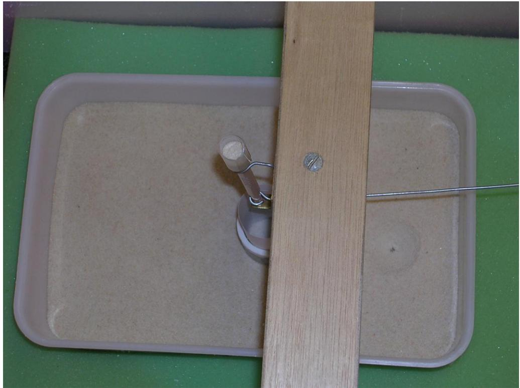
to deliver a vibratory cue, namely 4.5 mL of sand (approximately 5 s duration of vibratory cue). The sand fell into a sand-receiving container, which consisted of plastic wrap attached to the bottom of a 3.8 cm tall section of 1.5 inch PVC pipe, and which was placed underneath the delivery device. The sand-delivery device and the sand-receiving container were positioned so that the cue was delivered 4.5 cm from the center of the pit.
