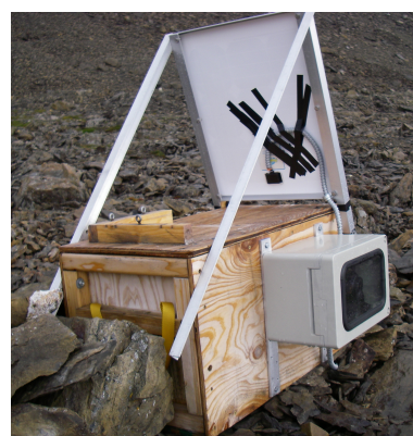
Figure 2: Plumecam case with solar panel
