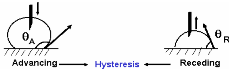
Figure 7. Measurement of advancing (left) and receding (right) contact angles
