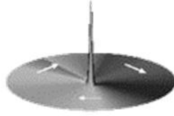
Figure 3: Perspective view of the magnetization of a clockwise vortex structure of a disk with moments popping out-of-plane to form a core due to exchange interaction of closely packed anti-parallel aligned moments at the center (Ref. [2])
