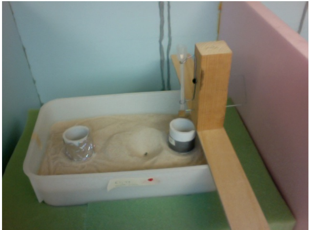
Figure 2. Top-view of the sound-attenuating apparatus, showing an antlion in its conical pit, the two collecting containers, and a wooden cue delivery device.
