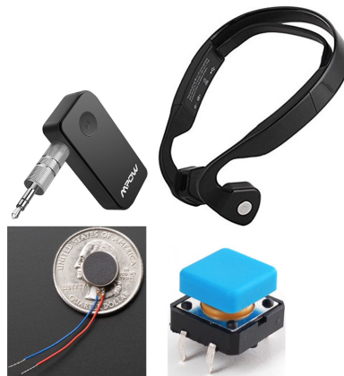
Figure 7: The audio and vibro-tactile user interface communicators. (Clockwise from top-left: Bluetooth transmitter, Bluetooth Bone-conduction headphone, Adafruit's vibrating mini-motor disk, and push button) [iii, iv]
