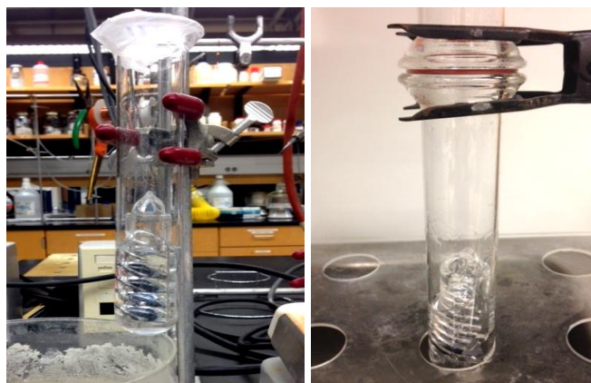
Figure 33: Preparation for protein adsorption studies by soaking in PBS prior to exposure to proteins (left). Incubation of the substrates in protein solutions (right).
