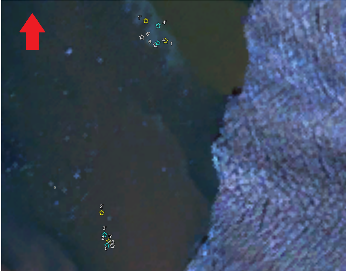
Figure 1: The lower cluster of drogues are in the delta region, and the upper cluster is in the upwelling overflow region. Drogues 1 to 6. 1 and 2 are in yellow, 3 and 4 are in blue, 5 and 6 are in white. The numbers indicate the starting point and the prime indicates the end point; for example, the yellow star labeled 1 is where drogue 1 was released; the yellow star labeled 1' is where drogue 1 was retrieved. Note that drogue 5 barely moved and has a much smaller velocity than the other surface drogues in the delta region; this might be due to daily variability in the delta discharge velocity (drogue 5 is the only surface, delta measurement for that day).
