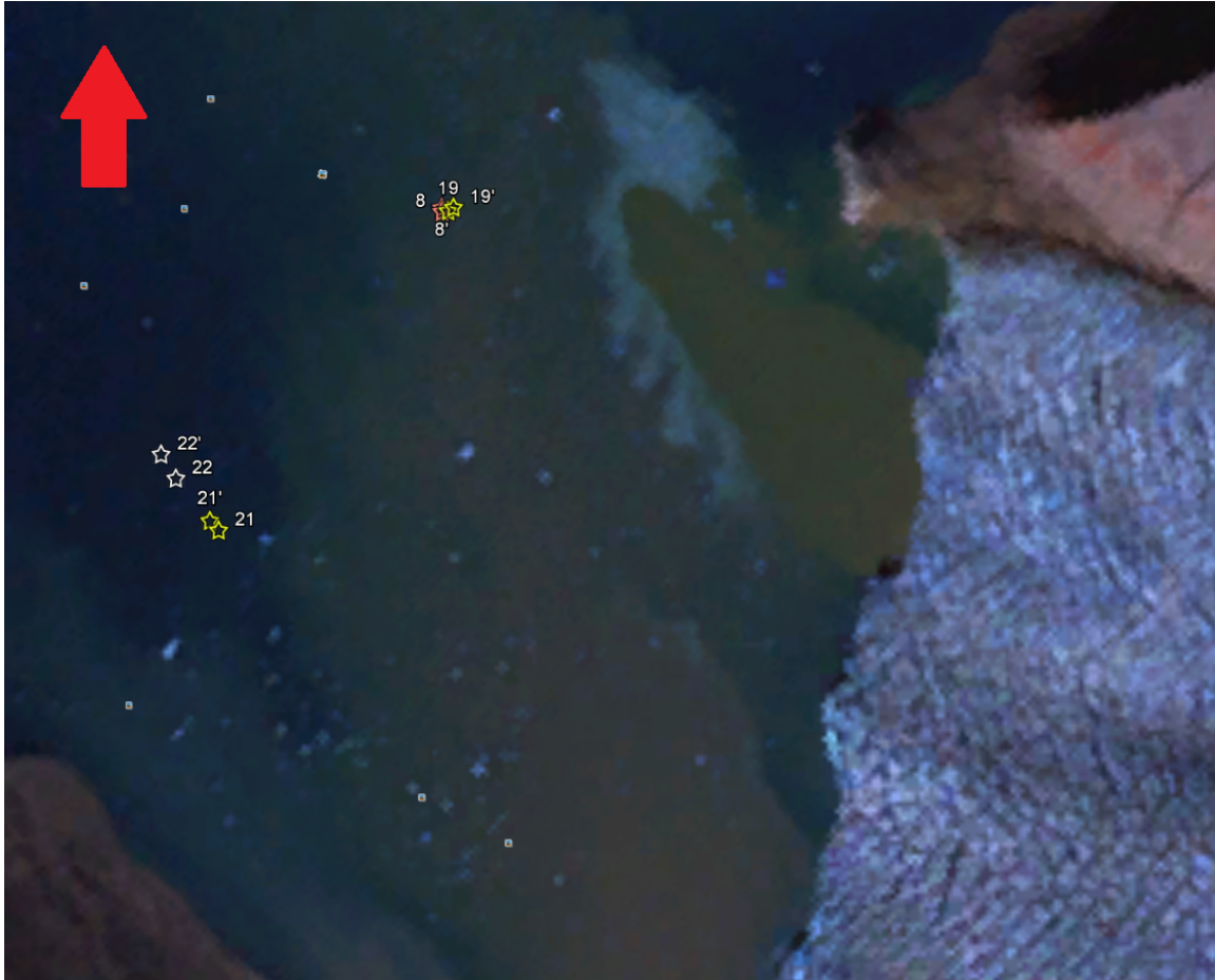
Figure 5: At 50 m depth, farther away from the ice face and at the centerline of the fjord, the water mass appears to be still (see drogue measurements 8 and 19, both at flood-tide). Along the southern shore of the fjord, the water is moving away from the ice face (see drogue measurements 21 and 22, both also at flood-tide). Drogue 8 is in peach, drogue 19 is in yellow. Drogue 22 is in white, drogue 21 is in yellow.
