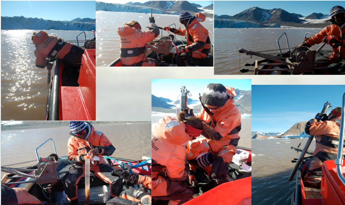
Figure 5. The gravity core collection process, clockwise from top left. (1) The corer is dropped into the water, (2) the corer is lowered to depth, (3) after impact, the corer is raised, (4) the corer is hoisted out of the water, (5) the core liner is removed from the barrel, and (6) the core is sealed.
