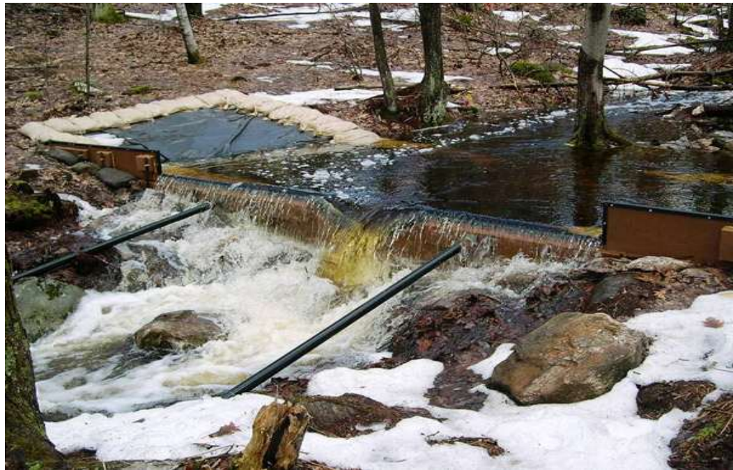
Figure 3. Big Weir in Nelson Brook at the Harvard Forest. At the bottom of the weir behind the barrier are placed pressure sensors. The shape through which the water flows is restricted by the barrier to be regular, allowing for the discharge to be calculated solely based on the input data for pressure. Photo by Emery Boose
