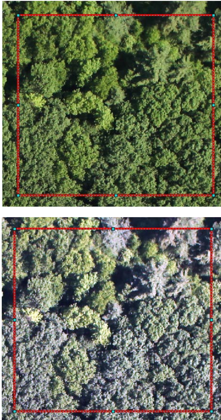
Figure 26a and b. Natural color (top) and standard deviation stretch (bottom) of an area within my study site. The stretch is one technique to help distinguish individual trees.
