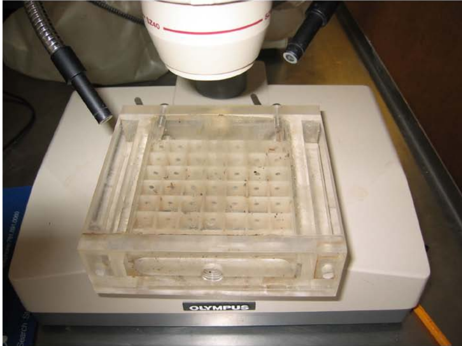
Figure 4. The synthetic crab fly chamber. The fly chamber is a square 9.5cm plastic grid inside a closed Lucite box. The chamber is detachable from the rest of the apparatus so that it can be placed under the microscope.
