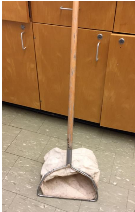
Figure 4. The D-Frame Net used in the dip net method for sampling the lake sites.
