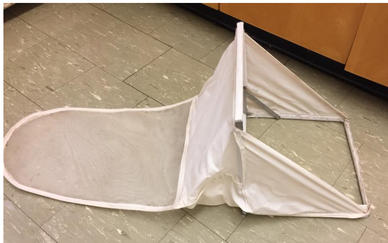
Figure 3. The Surber 500Mu Nitex Net used in the kick seine method for sampling the stream sites.
