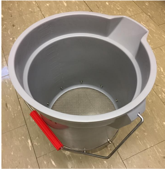
Figure 5. The sieve bucket used to strain collected sediment in the dip net method when sampling the lake sites.
