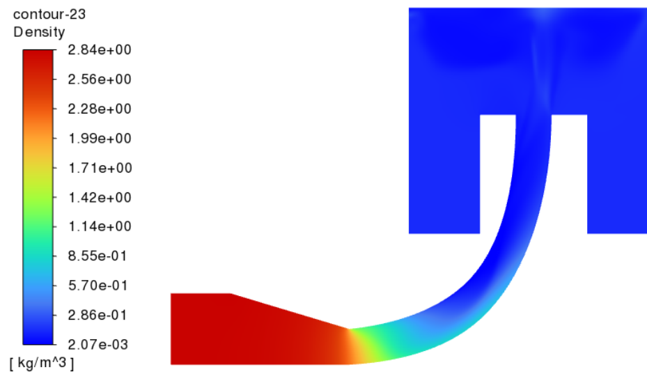
Figure A.3 Nozzle 1 density distribution.
