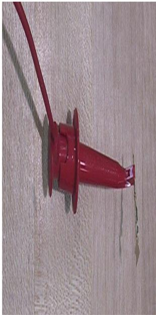
**Figure 52 – Probe used to test Thermocouple Resistance**
