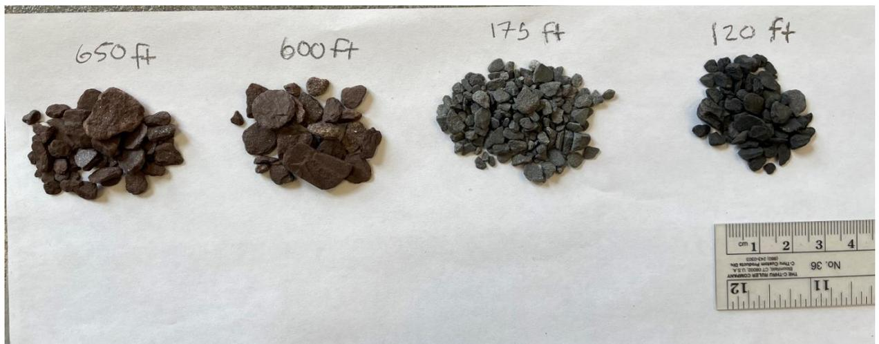
Figure 5. Samples of drill cuttings from various depths that show differences in color of the main stratigraphic units (120ft = dark gray; 175 ft = gray; 650 ft, 600 ft = red).
