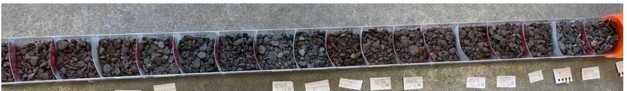
Figure 4. Composite made of drill cuttings. Section shows 295 ft – 370 ft of the 800 ft record (left to right).
