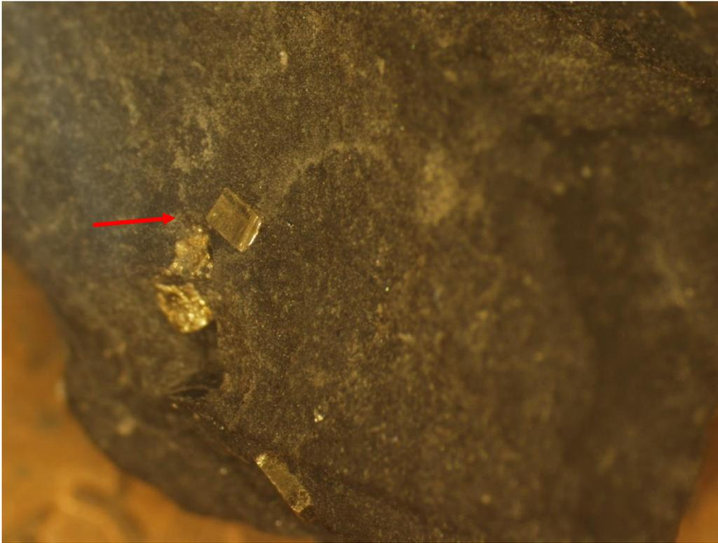
Figure 24. Pyrite crystals (1mm) in the dark gray shale on US penny. Shale chip is about 1 cm in length.
