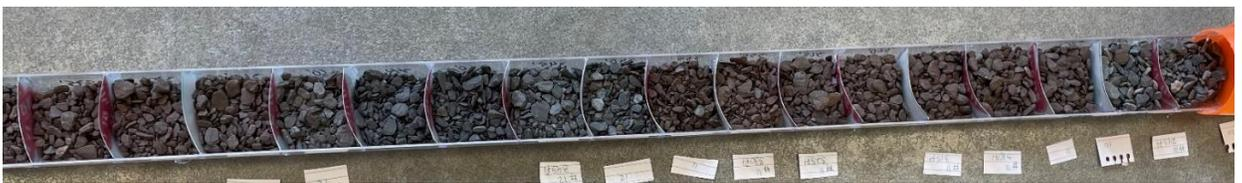
Figure 4. Composite made of drill cuttings. Section shows 295 ft – 370 ft of the 800 ft record (left to right).
