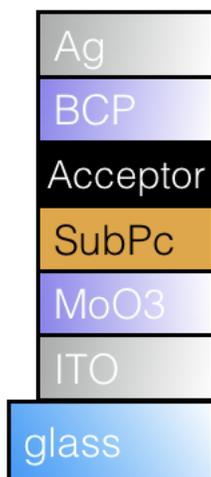
Figure 1-4: A Typical Solar Cell with SubPC as the Donor Layer
