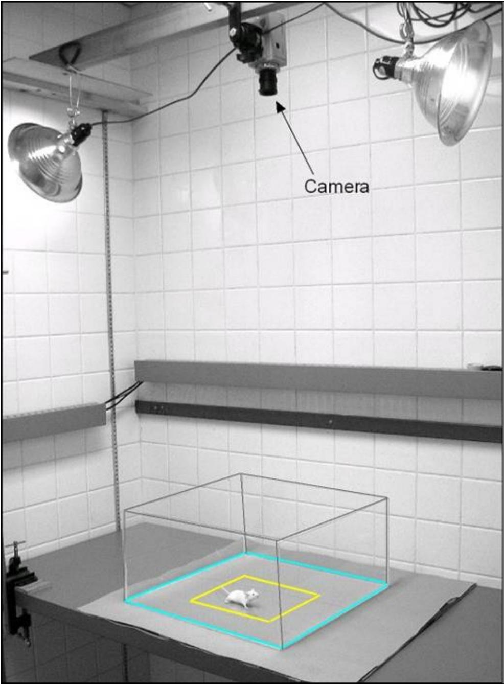
*Figure 2.* Light-dark box (40 [L] x 40 [W] x 20 [H] cm) used to assess fear in mice. Half of the box was covered with black cardboard to create distinct light and dark sections.
