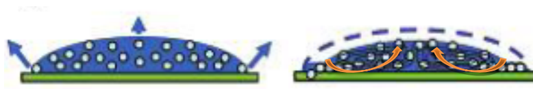
Figure 2. Cross-sectional view of the droplet profiles. Left: the nonuniform distribution of evaporation flux along the surface is represented by the length of the arrows above the droplets. Right: hydrodynamic flows generated by inward Marangoni effect (indicated by the orange lines). 8
