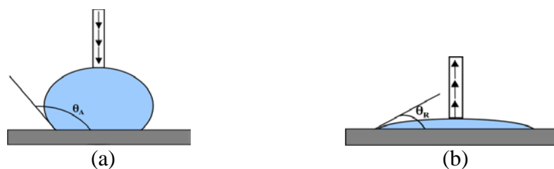
Figure 11. Measurement of dynamic contact angles: (a) an advancing angle and (b) a receding angle. 45
