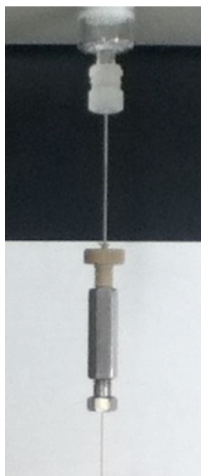
Figure 1.16. A steel and PEEK union connecting the needle of a syringe to a capillary
