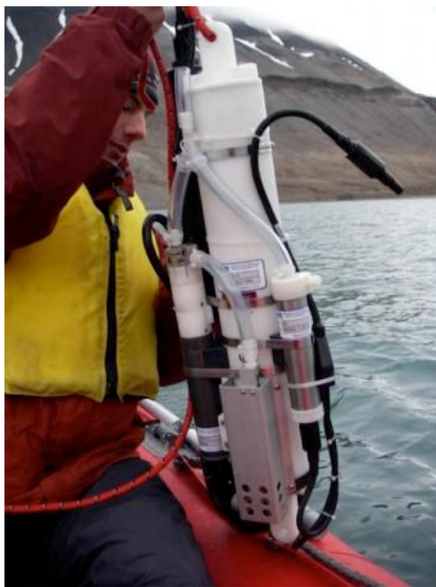
Figure 12. Vertical casts involved lowering the Seacat ® into the water column at mooring sites throughout the lake.
