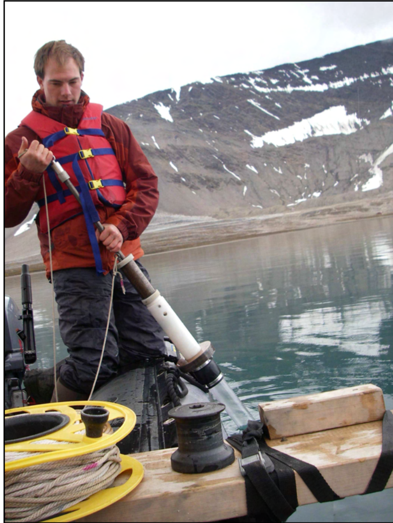
Figure 2.2: The author prepares to core during a calm day on Linnévatnet using the Universal Surface Corer.
