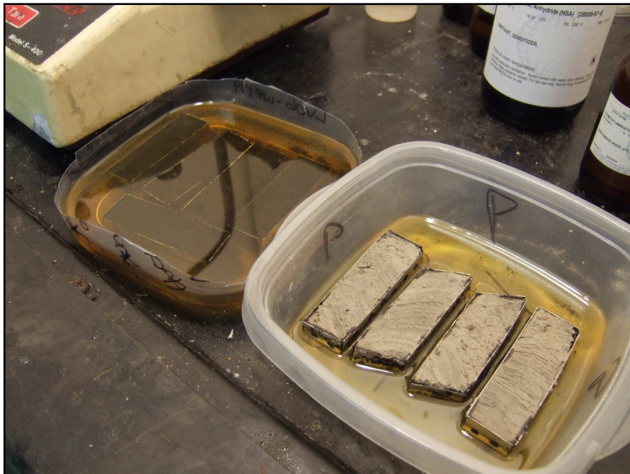
Figure 2.7: Freeze dried samples in epoxy impregnation stage. Tray on the left has otopped thin sections after saturation in the vacuum chamber; tray on the right is ready to go into the vacuum chamber.
