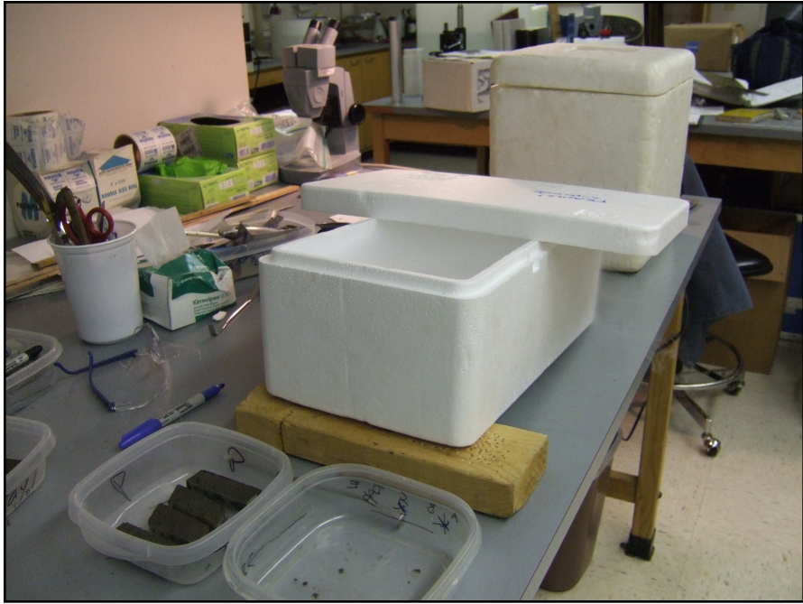
Figure 2.6: Setup for freeze drying thin section samples. Note trays of thin sections, inclined styrofoam box for initial freezing, and second box for longer submersion.
