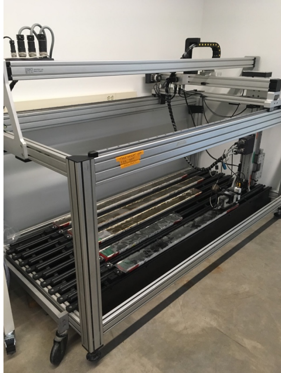
Figure 4. Geotek MSCL-XYZ point sensor taking MS measurements every 0.5 cm.
