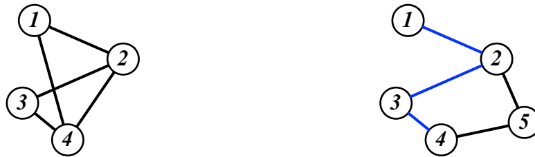
(a) An undirected graph with V = \{1, 2, 3, 4\} and E = \{12, 14, 23, 24, 34\} . (b) An undirected graph with a path between vertex 1 and 4 highlighted in blue.
