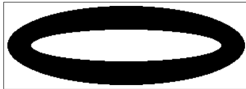
FIG. 1. Sample mask. The black portion is magnetized and white not magnetized. The black rectangular frame is added to show the mask boundaries and is not magnetized.
