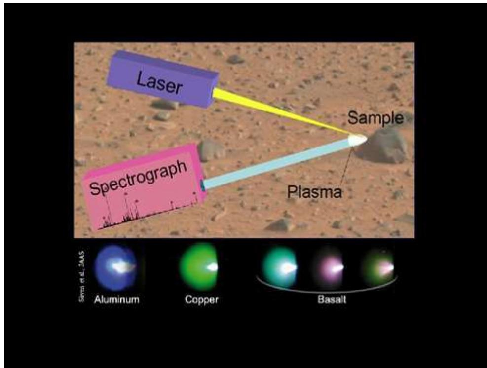
**Figure 2:** Schematic of laser-induced breakdown spectroscopy
