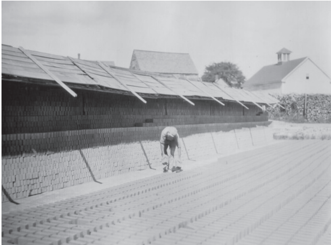
Bricks drying out in North Cambridge Brickyard, 1930s. Image from History Cambridge.
