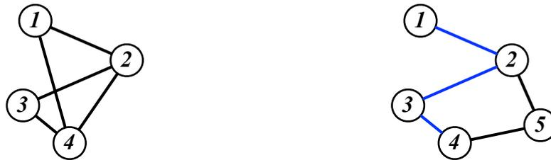
(a) An undirected graph with  $V = \{1, 2, 3, 4\}$  and  $E = \{12, 14, 23, 24, 34\}$ . (b) An undirected graph with a path between vertex 1 and 4 highlighted in blue.
