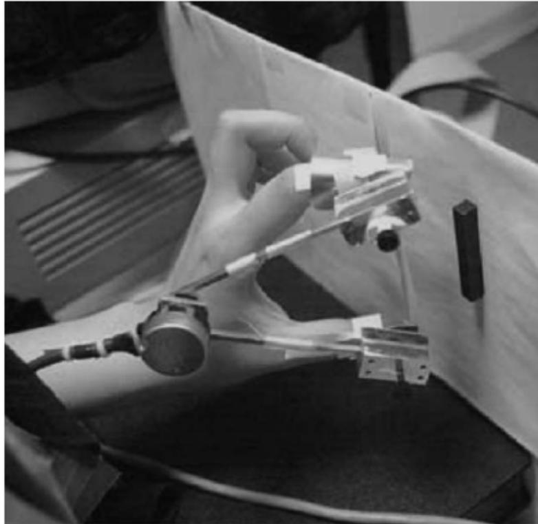
Figure 3. Optotrak (Northern Digital, Waterloo, ON, Canada) devices, with infrared light-emitting diodes attached to various points on the hand. (a) 3-marker method used by some researchers (e.g. Franz et al., 2000; Franz, Hesse, and Kollath, 2009) (b) 1-marker method in which single LEDs are attached to the index finger, thumb, and wrist, generally used in experiments by Goodale and colleagues (e.g. Aglioti et al., 1995; Goodale, 2008). Both images are from Franz, Hesse, and Kollath (2009).
