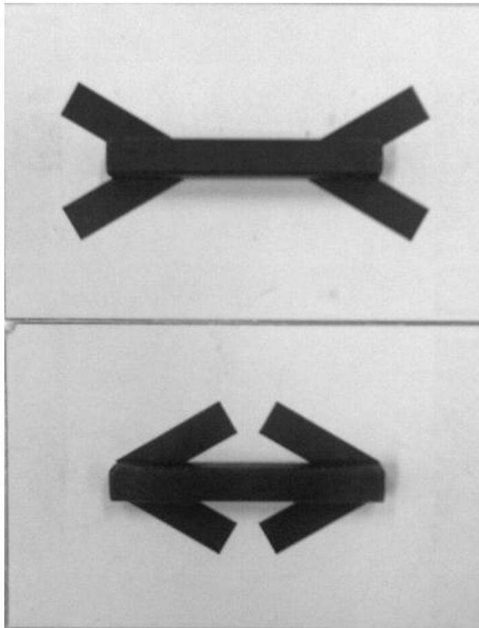
Figure 5. Our modified version of the recording device used by Radoeva et al. (2005). Like the original device, this device consists of a potentiometer, 12V power supply, two aluminum arms (thinner than on the Radoeva et al., 2005 device) and two finger-holders (now rubber bands). The voltage through the potentiometer was monitored by a computer via a National Instruments Data Acquisition Card (NI-DAQ-1200).
