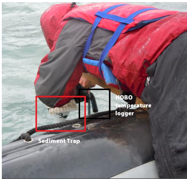
Figure 2.2: Mooring Line with both a Temperature logger and a sediment trap
