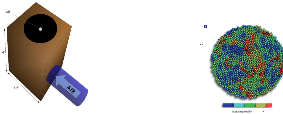
(a) Schematic of the experiment. The particles used in this system were steel spheres of two sizes, 0.318 and 0.397 cm.
