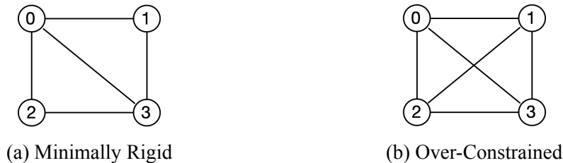
Figure 4: Minimally rigid (upon removal of any edge, graph is flexible) vs over-constrained (upon removal of an edge graph is still rigid)
