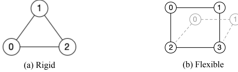
Figure 3: Rigid vs. flexible graphs. (a) is rigid because there is no way to alter any pairwise distances in the graph. (b) is flexible because if e_{01} is moved, the pairwise distance between v_0 and v_3 changes and the pairwise distance between v_1 and v_2 changes.
