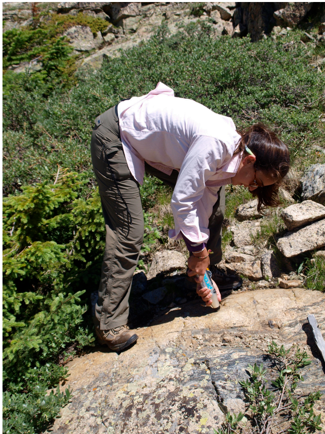
Figure 16: The author operating the Schmidt Hammer in the Green Lakes Basin field area (Image from: D. Dethier).
