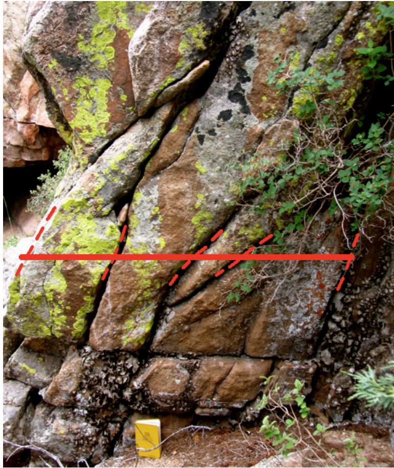
Figure 17: The solid red line represents the measuring tape that was held parallel to the ground and straight along the tor. The smaller dashed red lines indicate fractures where a measurement would have been taken. The measuring transect would both begin and end at a fracture plane.
